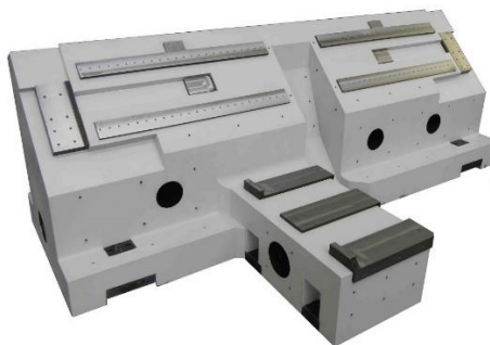
Figure 1. lathe bed from Ultra-High-Performance Concrete (UHPC) [8]
