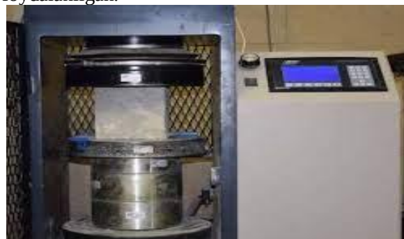
5-rasm. YES-2000 Betonni siqish sinov mashinasi
